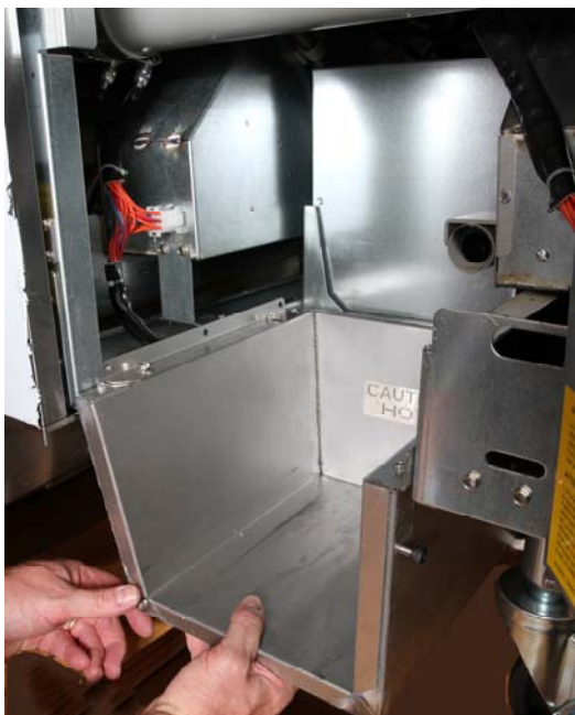
Figure 2: Position the melter.
